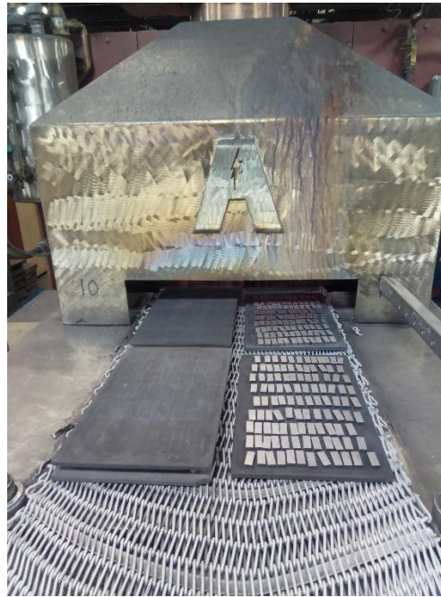
Figure 5. Photo of TRS samples loaded on the conventional sintering furnace.
