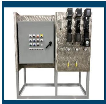
Industrial furnace atmosphere panels play a critical role in processes where maintaining a specific furnace atmosphere is essential to the material's quality and performance, such as heat treating, sintering, and metal finishing.
