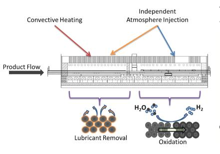
Lubricant is required for the compaction of the powder metal component; however, if all of the lubricant is not removed prior to applying the oxide coating, carbon soot from the lubricant will contaminate the oxide coating and negatively effect the magnetic properties of the final component.
