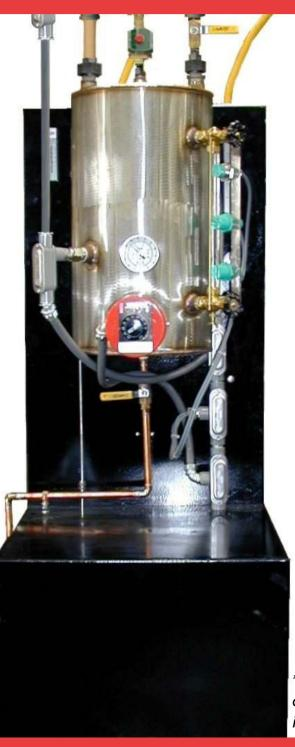
The MIS100 is designed to inject a watermisted stream of nitrogen into a continuous furnace to increase the dew point. Typically, the MIS100 will deliver approximately 6 lbs. of water/hr\*.
