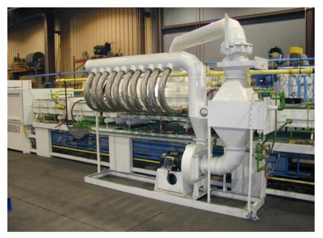
Convective cooling is recognized as a method of improving metallurgical properties without subsequent heat treating processes. Abbott Furnace Company's VariCool System combines radiant and convective cooling to accelerate the cooling capabilities of continuous belt furnaces. Available on all new continuous furnaces, the VariCool System can also be retrofitted to existing furnaces.
