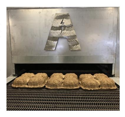
The ability to control timing (i.e., travel speed), temperatures, atmospheric moisture levels, and airflow is critical in oven design. It is also important that these factors can be adjusted easily to accommodate a variety of shapes, sizes, of molded pulp products.
