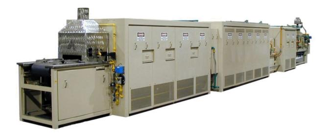
**Solving manufacturing challenges with a redesigned sintering furnace** One of the biggest challenges with soft magnetic composites is removing the lubricant completely and efficiently from the compacts. Conventional sintering furnaces are used for this; however, they risk heating the parts too quickly or too hot, which creates damaging soot. Lower temperatures avoid the sooting but often require multiple passes through the furnace, which slows the manufacturing process.
